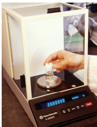
A Figure 1.10A This balance is accurate to 0.01 g
