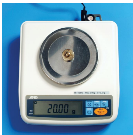
A Figure 1.10A This balance is accurate to 0.01 g
