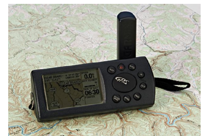
Figure 1.28 A GPS (Global Positioning System) receiver
